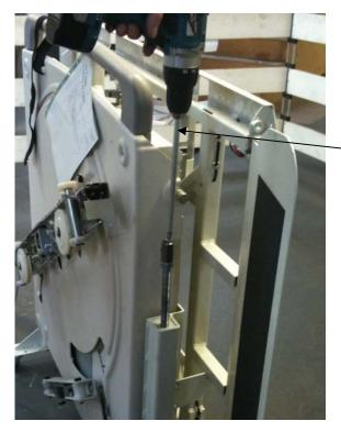
Jack height adjustment made by a battery drill and emergency release tool bar or 24mm socket
